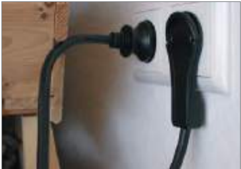
Extremely flat plug fit; plug protrudes from the socket by just 7 mm.
